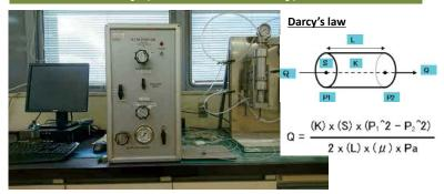
Permeability is an indicator of the ability for oil and gas to flow through the pore space of a rock.
