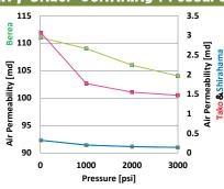
In oil and gas reservoir, overburden (confining) pressure affects porosity and permeability. Porosity and permeability under confining pressure are also usually measured in our laboratory.
