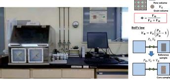
Pores are void spaces in rock and are measured as porosity, which is the fraction of the volume of void space over the total volume of the material.
