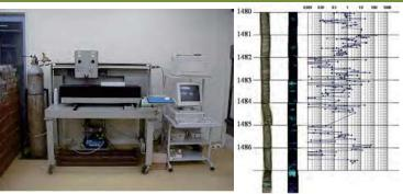
The permeability of the rock (whole core) surface is measured simply and sequentially.
