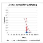
The permeability of each reservoir fluid, such as oil or gas, correlates with the saturation of that fluid in pores. This property is called the relative permeability and is estimated from the results of a core flooding test performed at reservoir conditions.
