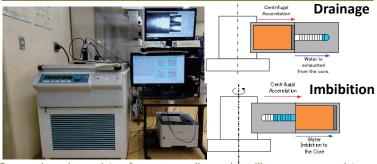
Reservoir rock consists of porous media, and capillary pressure exists between different fluids, such as oil and gas, in those media. Capillary pressure affects fluid flow and saturation in a reservoir and is often measured using a centrifuge.
