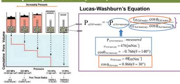
MICP (mercury injection capillary pressure) is used to measure the capillary pressure of samples too small or brittle to core.
