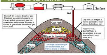
An oil and gas deposit consists of fine-grained rock (called the cap rock), which acts as a lid, and reservoir rock, which holds oil and gas within its pore space. Estimation of the rock properties of an oil/gas reservoir is crucial to development of that reservoir.
